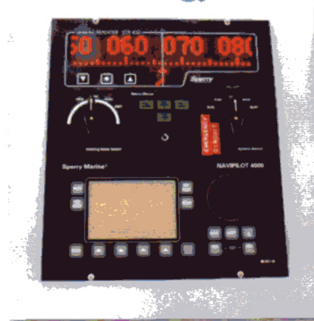
The Sperry Navpilot 4000 steering stand on the Hon. James L. Oberstar is tied to the ship's gyrocompass.
