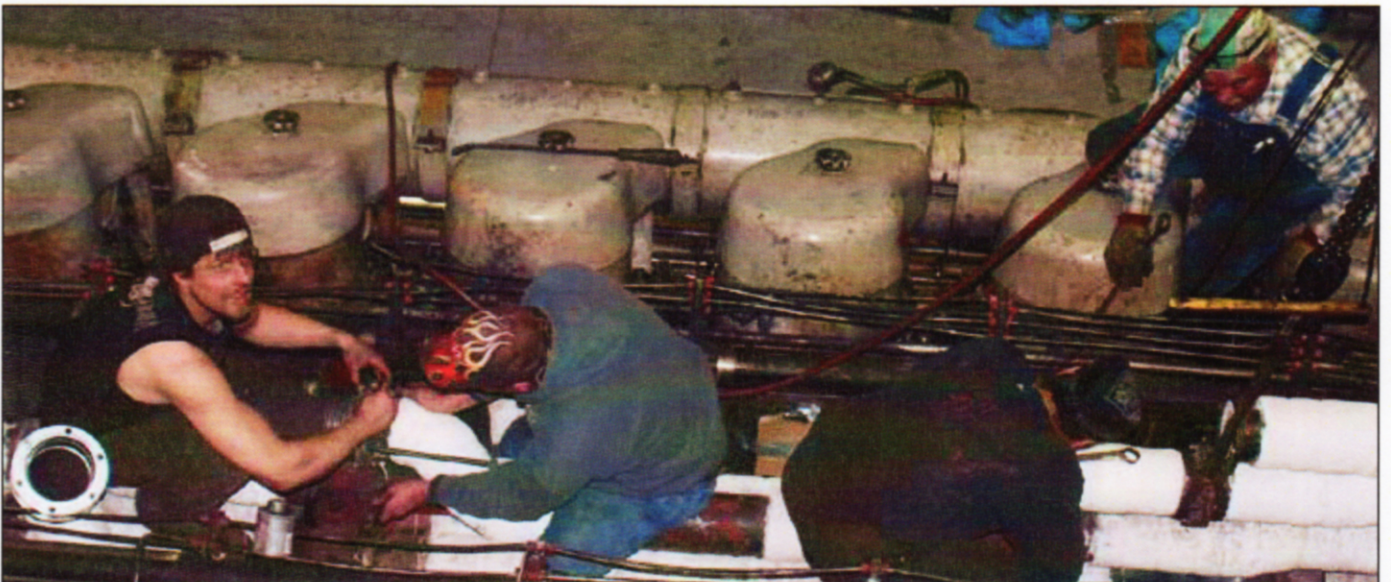
Fraser Shipyards crew reassembles an engine exhaust system after overhauls.
