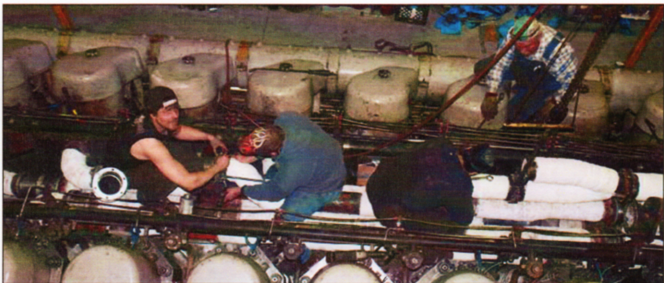
Fraser Shipyards crew reassembling an engine exhausts system after engine overhauls
